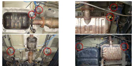
Figure 2 Test setup for measuring the acceleration of vehicle body and exhaust system.
