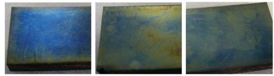
Fig. 7. State of coating layer after 120 times thermal shock test
