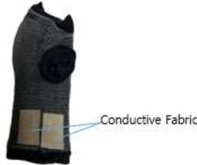
**Figure 12.** Attaching Conductive Fabrics (taken by author)
