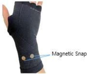
**Figure 11.** Attaching Conductive Snaps (taken by author)
