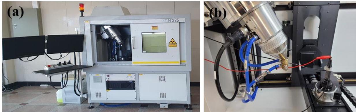
Figure 1. (a) Nikon XTH 225 system, and (b) X-ray beam generation unit.
