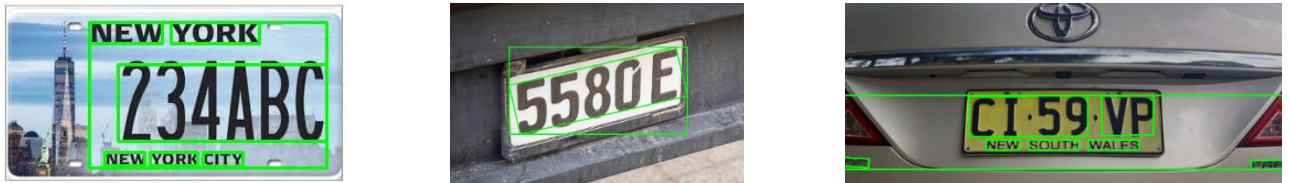
Figure 8. Vehicle license plate recognition through OCR
