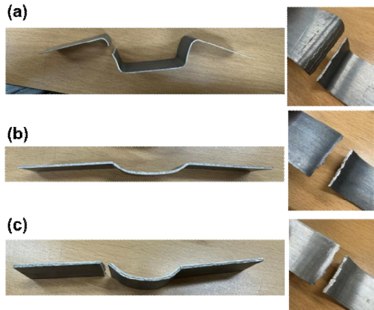
Fig. 13 Pictures of the fractured specimens with different thickness values (a) 1 mm, (b) 2mm, and (c) 3mm
