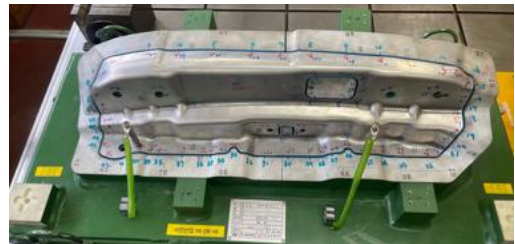
Fig. 7 Die Process Result & Checking Fixture.
