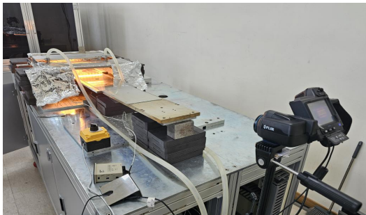
Fig. 6 Curved glass thermal molding system using self-weight
