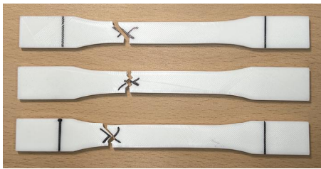
Fig. 6 Specimen broken after the tensile strength test of the specimen output by applying the printing condition with the highest tensile strength value
