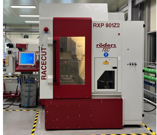
Fig. 1 High-speed precision machining 3-axis cnc machining center (RXP 801 Z2, rodgers)
