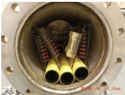
Fig. 7. Materials soaking chamber
