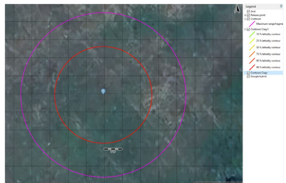
Fig. 8. Lethality range and maximum fragment range caused by explosion overpressure
