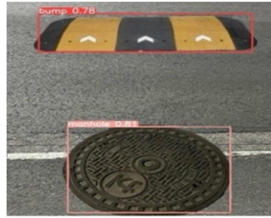
(b) bump and manhole Fig. 2. Detection results screen
