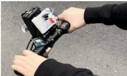
Fig. 9. Appearance of the final warning device for personal mobility
