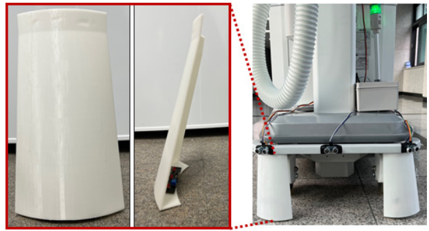
(a) Supporter of three-channel infrared line tracer sensor
