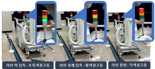
(b) Color change of warning light by 3-channel infrared line tracer sensor
