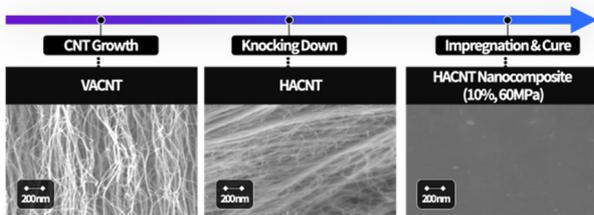
Fig. 5. Cross-section image of specimen at manufacturing stages
