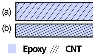
Fig. 9. Schematic diagram of VACNT according to compression (a) HACNT Nanocomposite under low pressure, (b) HACNT nanocomposite under high pressure
