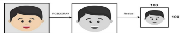
Fig. 3: Conversion of a RGB image to a Gray Scale image of 100 x 100 size [8]
