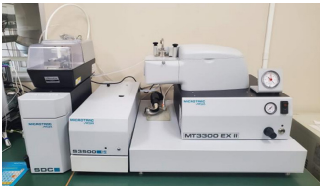
Fig. 2. Experimental apparatus for measurement of dust particle size and distribution.
