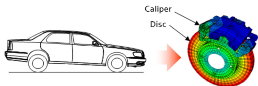
Fig. 1 Schematic of braking heat generation
