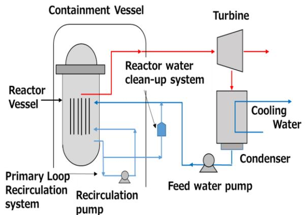
Fig. 4. Schematic diagrams of BWR.
