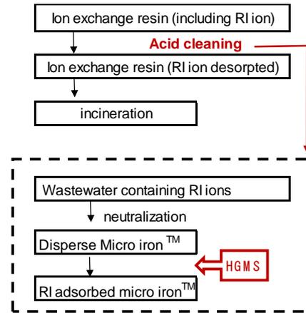
Fig. 5. Flow chart of used ion exchange resin processing, After acid cleaning, High Gradient Magnetic Separation (HGMS) will be used.
