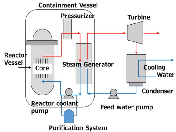
Fig. 3. Schematic diagrams of PWR
