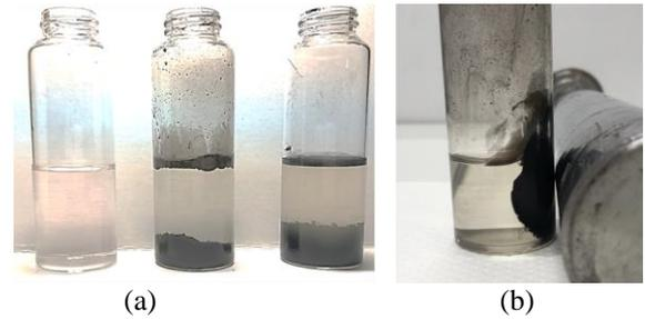
Fig. 8. Adsorption of cobalt ions and magnetic separation of the adsorbent. (a) From the left, cobalt aqueous solution, adsorbent dispersion, and magnetite dispersion. (b) Magnetic separation of the adsorbent after cobalt adsorption.
