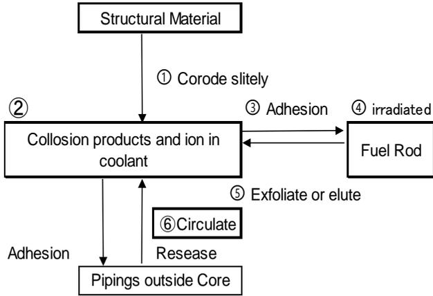
Fig. 1. Radioactivity accumulation mechanism in Primary Cooling System
