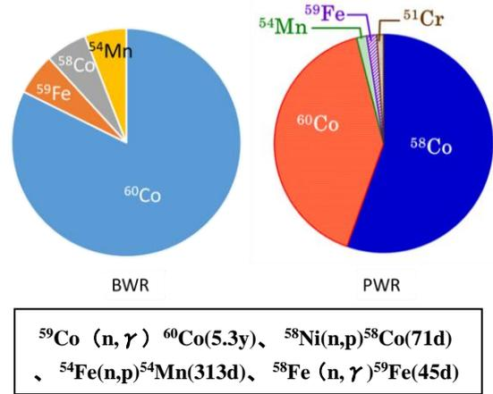
Fig. 2. Radionuclides in the crud together with the nuclear reactions in which they are produced.
