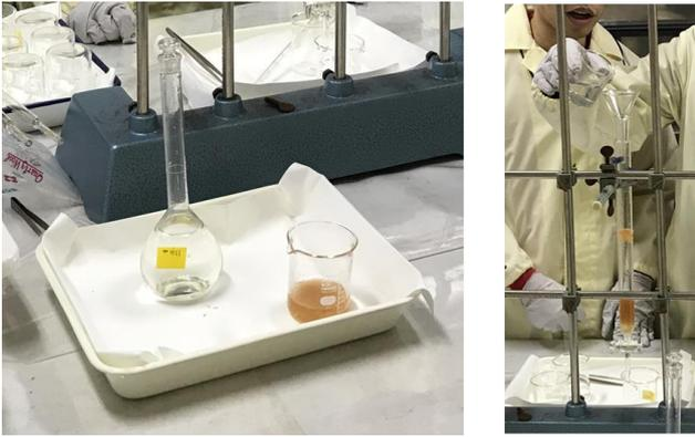
Fig.6. Adsorption and desorption test of cobalt-60 using ion exchange resin.
