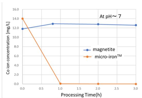
Fig. 7. Comparison of the adsorption efficiency of cobalt ions between adsorbents and magnetite.
