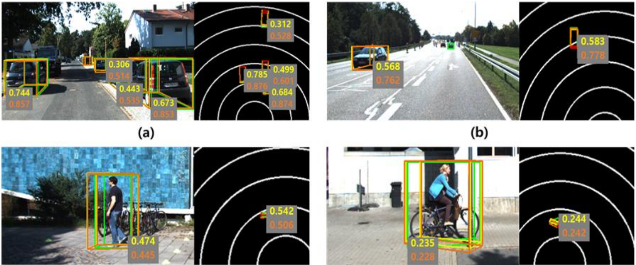
Fig. 4. KITTI Qualitative Results Examples. We visualize M3KD and PKD methods on the KITTI validation dataset. The orange, yellow, and green boxes in the image represent the 2D and top view projections of the predicted 3D bounding boxes of M3KD, PKD, GTs, respectively. Points side of boxes are 3D IoU and top view IoU points. The radius difference between two adjacent white circles is 5 meters.
