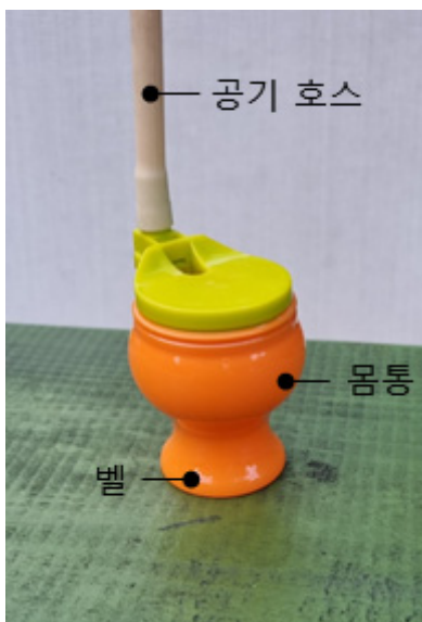
Fig. 2. Main components of the palm flute used for constructing the breathing excise musical instrument (BEMI).
