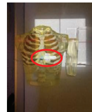
(c) Measuring method of ESD in left breast. The dosimeter was horizontally attached between the left 5th-6th thoracic spine of the chest phantom.
