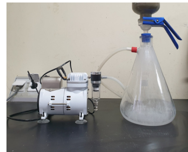
Figure 5. Apparatus for pore water extraction via vacuum filtration
