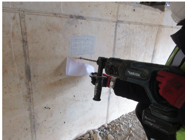
Fig. 1. Overview of carbonation depth test
