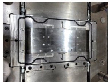
Fig. 13 Movable mold with EGI core pin and O-ring groove
