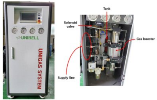
Fig. 11 Compressed air supply device
