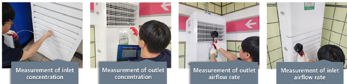
Figure 1 Measurement of collection efficiency and airflow rate of the air cleaner installed in the subway platform
