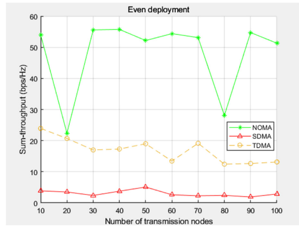
Fig. 7. Sum-throughput measurements based on the number of evenly deployed transmitting nodes.
