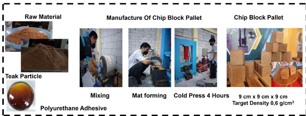
Fig. 1. Manufacturing illustration of chip block pallet.
