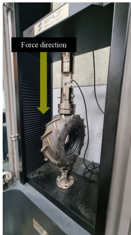
Fig. 6. Tire radial stiffness measurement using universal material tester.
