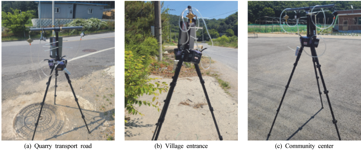
Figure 4. Installation of monitoring equipment for airborne dust at each measurement point
