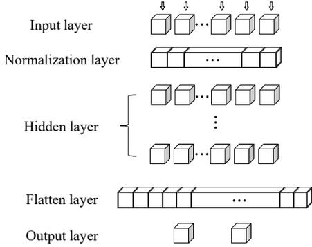
[Fig. 2] LoS/NLoS identification model scheme
