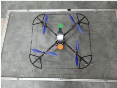
Figure 4: A quadcopter with attached two (green and red colored) AR markers on the frame body
