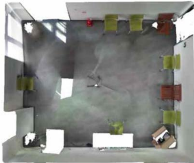
Fig. 3. Result of total indoor space point cloud extraction.
