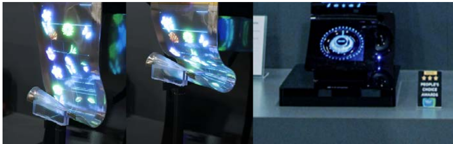
Fig. 1. LG Stretchable Display demonstrated at the Society for Information Display (SID) (Left) Demonstration of freeform deformation, (Right) Prototype covered on the multi-curved surface of an object
