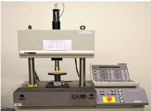
Fig. 6. INSTRON 8511 experimental device
