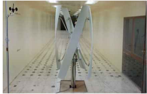
Fig. 9. Brake operation Test in wind tunnel
