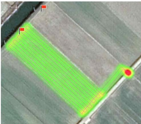
Fig. 8. Example of a pesticide control drone travel route in this study
