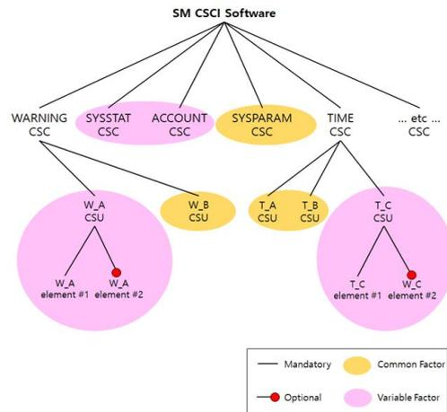
Fig. 3. Feature Model of System Management CSCI Software
