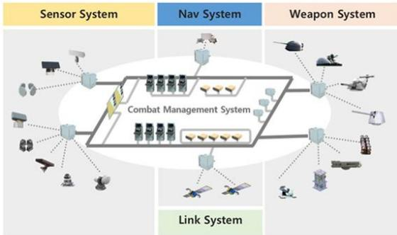
Fig. 1. System Architecture of Naval Combat Management System
