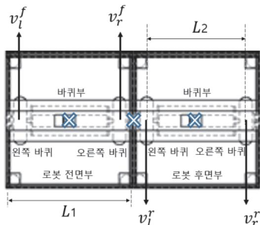
Fig. 8 Three centers of rotation of the robot
