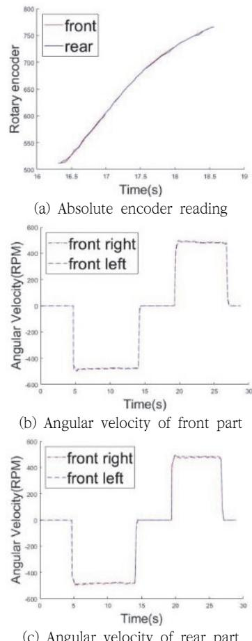
Fig. 10 Encoder outputs and angular velocities of the four wheels
