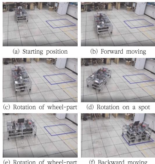
Fig. 11 Parking motion with rotation on the center of the robot body
