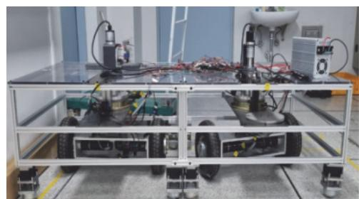
Fig. 1 The proposed four-wheeled mobile robot
