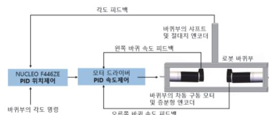
Fig. 5 Position control for wheel parts
