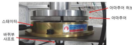
Fig. 3 Electric brake
