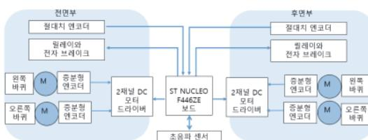
Fig. 4 Robot controller
