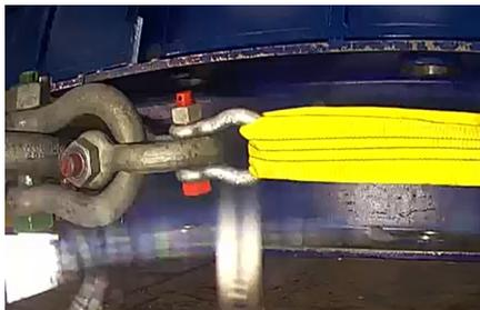
Fig. 1. Connection method of shackle and round-sling for breaking strength test.
