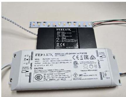
Fig. 7. DC24 V LED convertor & Zigbee controller.
