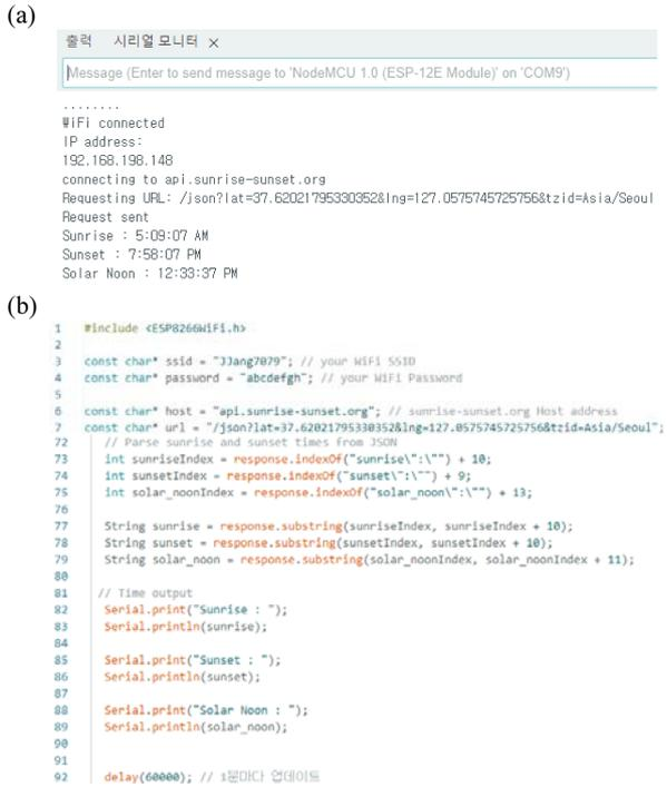
Fig. 10. (a) Serial monitor output result of Arduino sketch and (b) serial monitor output result of Arduino sketch.
