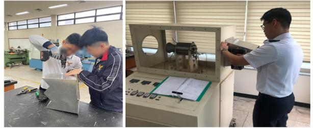
Fig. 5 Activities for chevron nozzle manufacturing and mounting on SR-30 turbojet engine apparatus
