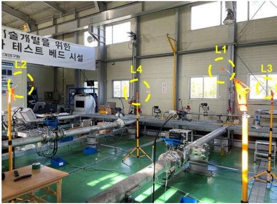
Fig. 3. (Color available online) Installation of virtual leakage sound sources.
