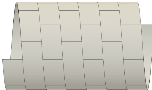
Fig. 1. Helical segment applied for consecutive shield TBM
