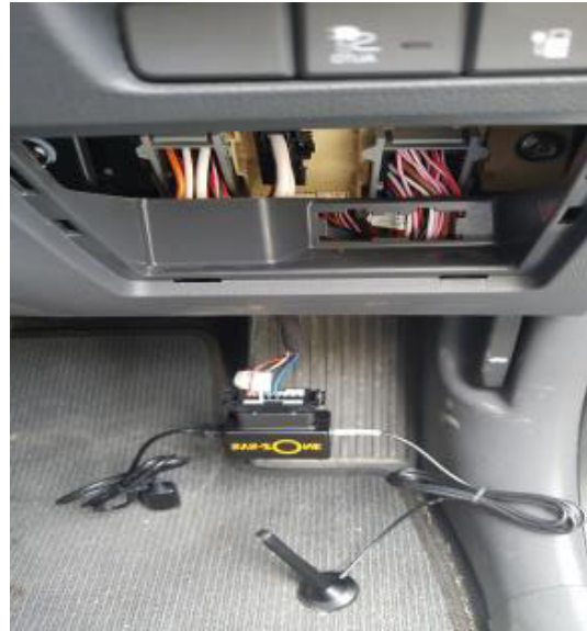
Fig. 2. Electric vehicle OBD installation.
