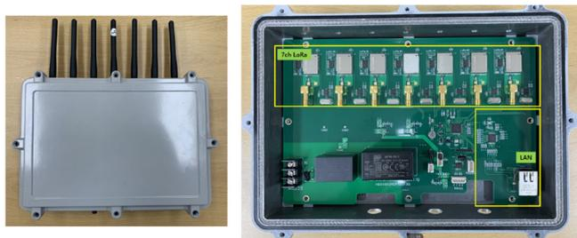
**Fig. 3.** Internal structure of Multi-channel repeater
