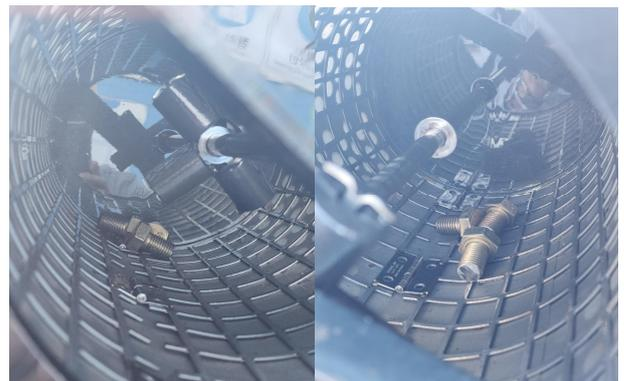
Fig. 13. Foreign substance bolt recovering from the filter after the impulsive operation.
