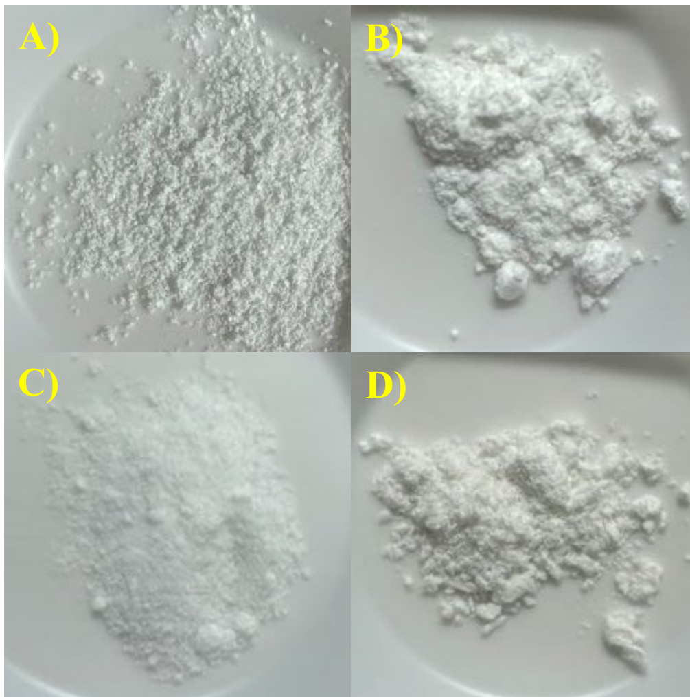
Fig. 3. Appearance of silodosin-loaded solid dispersions: (A) silodosin, (B) surface-attached solid dispersion, (C) solvent-wetted solid dispersion, (D) solvent-evaporated solid dispersion.
