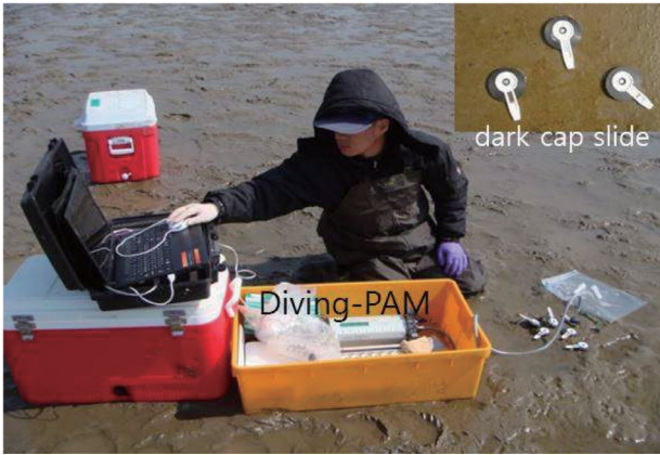
Fig. 2. Measurement photosynthesis of benthic microalgae by Diving-PAM and dark cap slide in the estuary of the Nakdong River.
