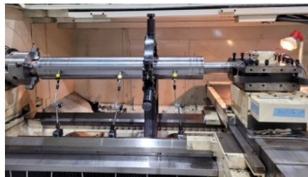
Fig. 10 Attachment of boring jig
