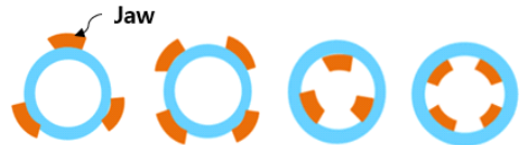
Fig. 1 Support conditions for outer-cylinder machining
